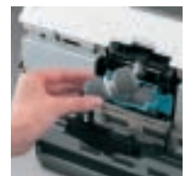
User-replaceable feed rollers
